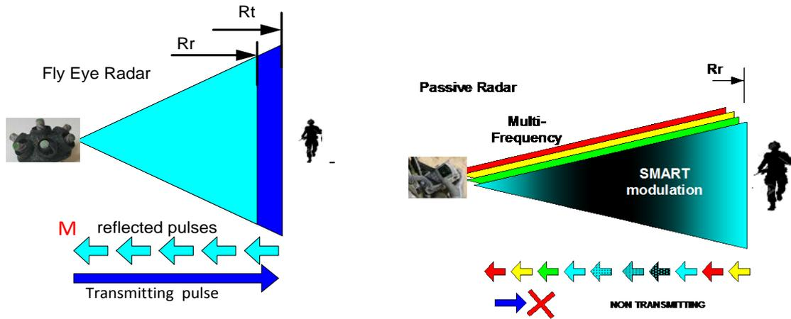
Figure 4. Range of detectable target \$R\_r\$ for Fly Eye radar. Passive regime of Fly Eye radar. Multi-frequency receiver with integration and smart modulation in each channel. Spectrum signatures provides possibility of automatic detection and recognition of different objects: human, small drones, weapon, explosives and different chemicals.
