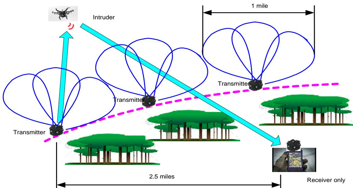
Figure 6. Transmitting modules can be distributed around perimeter of protected zone in bi-static drone detection system.
