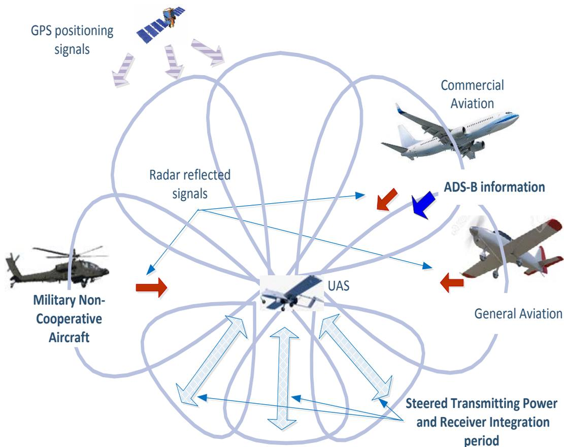
Figure 5. Ground clutter can be automatically suppressed in multibeam monopulse sense and avoid system by steering of transmitting power and receiver integration period in separate beams. System can be multi-function and combined with ADS-B system.
