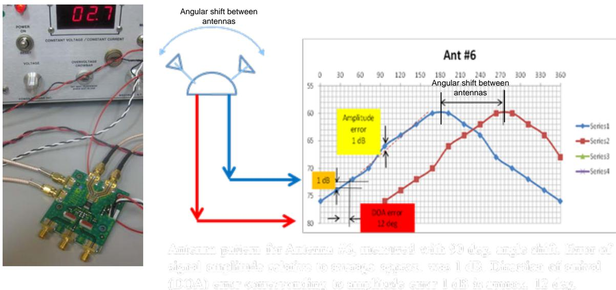
Figure 8. Test and accuracy estimation for direction finder with two directional antennas.
