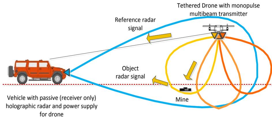
Figure 7. Mine detection from tethered drone provided possibility to detect mines 8-12 hours. Radar position optimal for mine detection.
