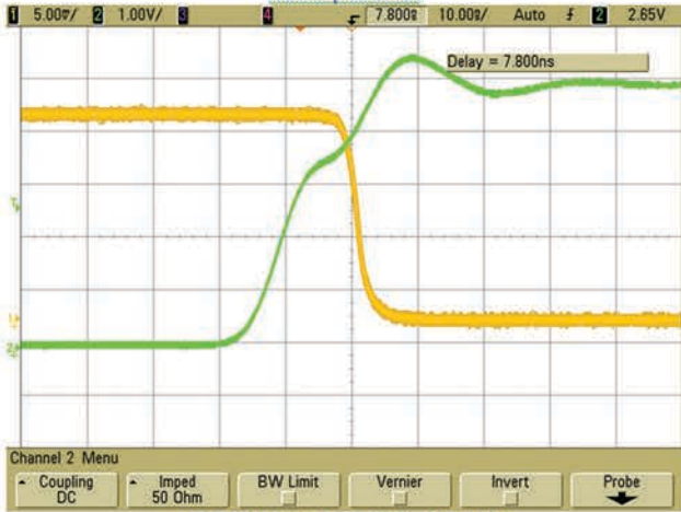
GREEN TRACE: TTL SIGNAL YELLOW TRACE: RF SIGNAL
